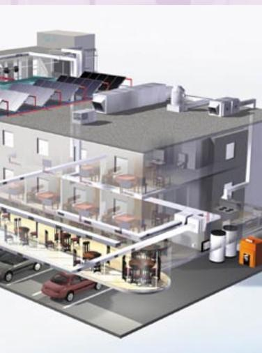
Passive House design would have a dramatic impact on energy conservation. A Passive House is a very well-insulated, virtually air-tight building that is primarily heated by passive solar gain and by internal gains from people, electrical equipment, etc. Energy losses are minimized. Any remaining heat demand is provided by an extremely small source. Annual energy requirement 15 kWh/m<sup>2</sup>/year.
